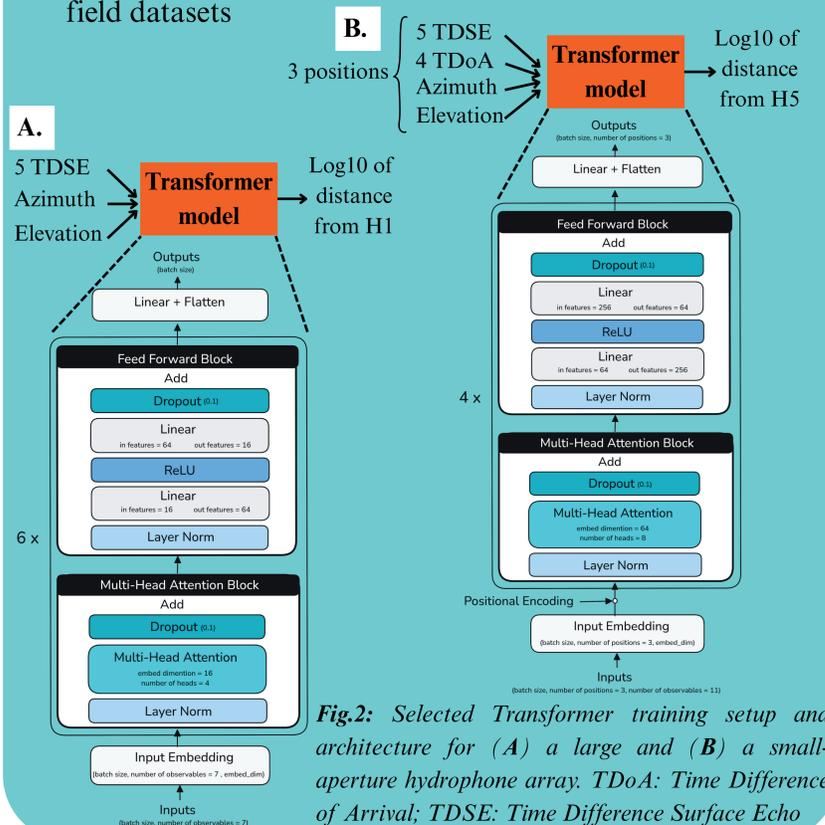
Fig.2: Selected Transformer training setup and architecture for (A) a large and (B) a small-aperture hydrophone array. TDoA: Time Difference of Arrival; TDSE: Time Difference Surface Echo
