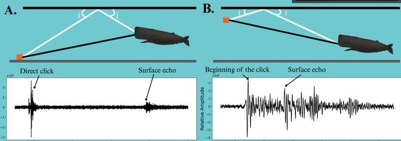
Fig.1: Surface echoes in case of (A) large and (B) small-aperture hydrophone array
