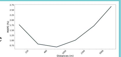
Fig. 3: MAPE on the simulated test dataset for the large-aperture antenna across different distance ranges
